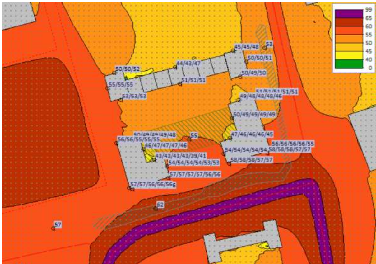
Figure 5 Daytime Period Noise Level Emission Contour Map (1.5m Height)
